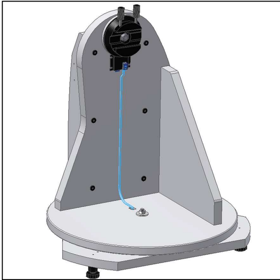
Figure 15. Install the supplied cable (part 4). A “click-sound” is heard when the socket connects correctly.
